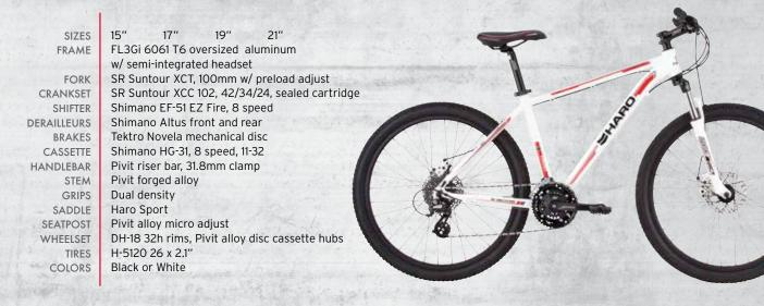
As the most affordable Haro mountain bike with disc brakes, the Flightline Two is a terrific choice for those looking to get big stopping power without a big price tag. Not only can it stop fast, but the 24 speed Flightline Two also boasts a lightweight FL3Gi aluminum frame, faster rolling tires and new graphics package. Crisp shifting plus stopping on a dime equals rave reviews for the 2013 Flightline Two. Available in four sizes.
