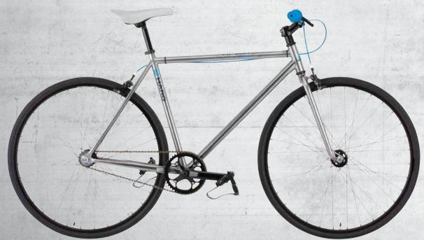
49cm, 53cm, 57cm Haro steel fixed gear w/ horizontal dropouts FRAME Full crmo FORK 4130 3 pc. tubular crmo w/ sealed BB/ 44T sprocket CRANKSET Tektro dual pivot caliper BRAKES CASSETTE 16t cog w/lockring Alloy riser bar; 70mm rise, 600mm Haro BMX alloy front load 52mm HANDLEBAR STEM Counterfeit BMX GRIPS Haro Slim padded SADDLE Steel 25.4mm SEATPOST 32H Weinmann XP26 alloy double wall; alloy flip flop Kenda Kwick Trax 700 x 38c WHEELSET TIRES Pearlple or Matte Black COLORS
