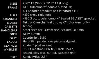
Taking it to the park or pump track, the Steel reserve 1.1 is the weapon of choice. Featuring an integrated internal head tube and full 4130 chromoly suspension corrected frame, forks and cranks, the Steel Reserve 1.1 can handle as much abuse as you can deliver while still possessing the light and agile qualities of a legendary Haro BMX bike.
